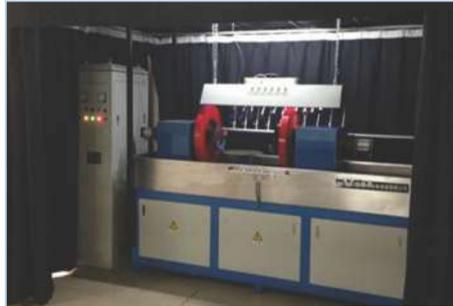
MPI (For Crack Check)
